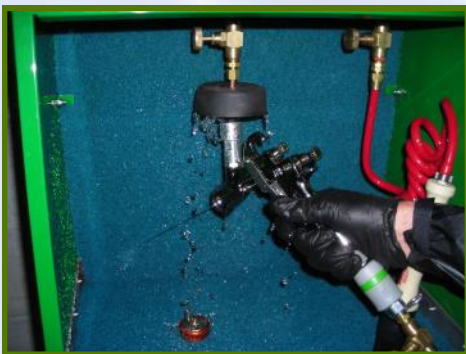
POWERPISTOL™ - Pulsating Fluid... Powerful Cleaning for the Fluid Passageways
